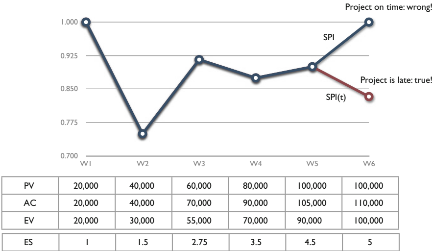
Fig. 12.8 The SPI and SPI(t) graph for the 5-activity example project
